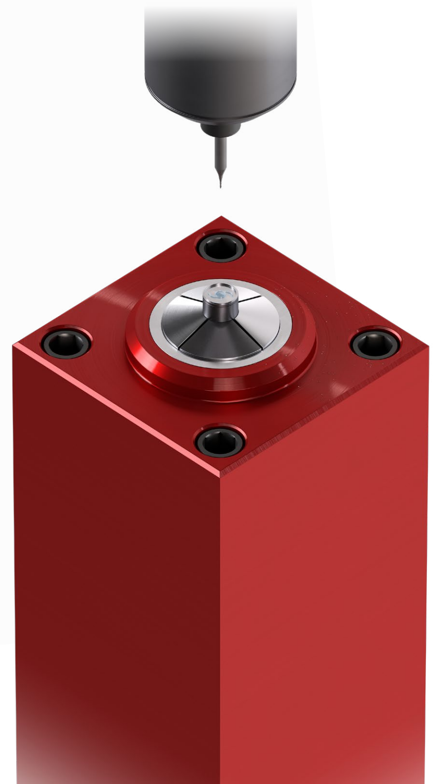
IOL in a Special Machining Jig
