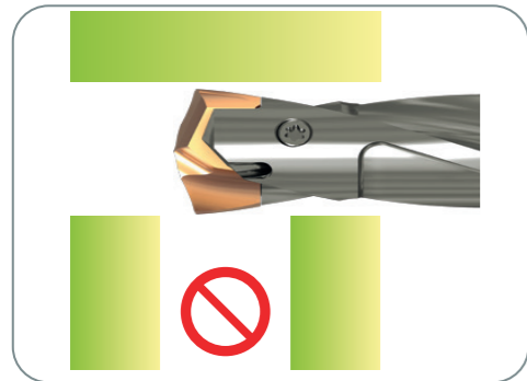
Intersecting cross hole is bigger than the drill insert's Margin Length.
